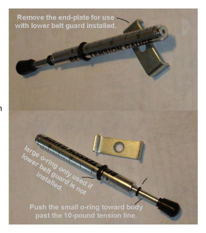
lower chain guard, or use the increments on the gauge.
