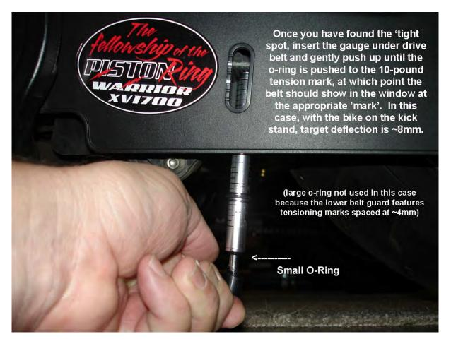
Once that is recorded, leave the bike on the ground and bounce it on its suspension a couple times to free the suspension after having been up in the air, then check belt tension again. This will highlight any difference, and understanding this will be handy one day when you're riding and anxious about your belt's condition.
