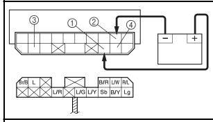
Does the starting circuit cut-off relay have continuity between blue and blue/white?
